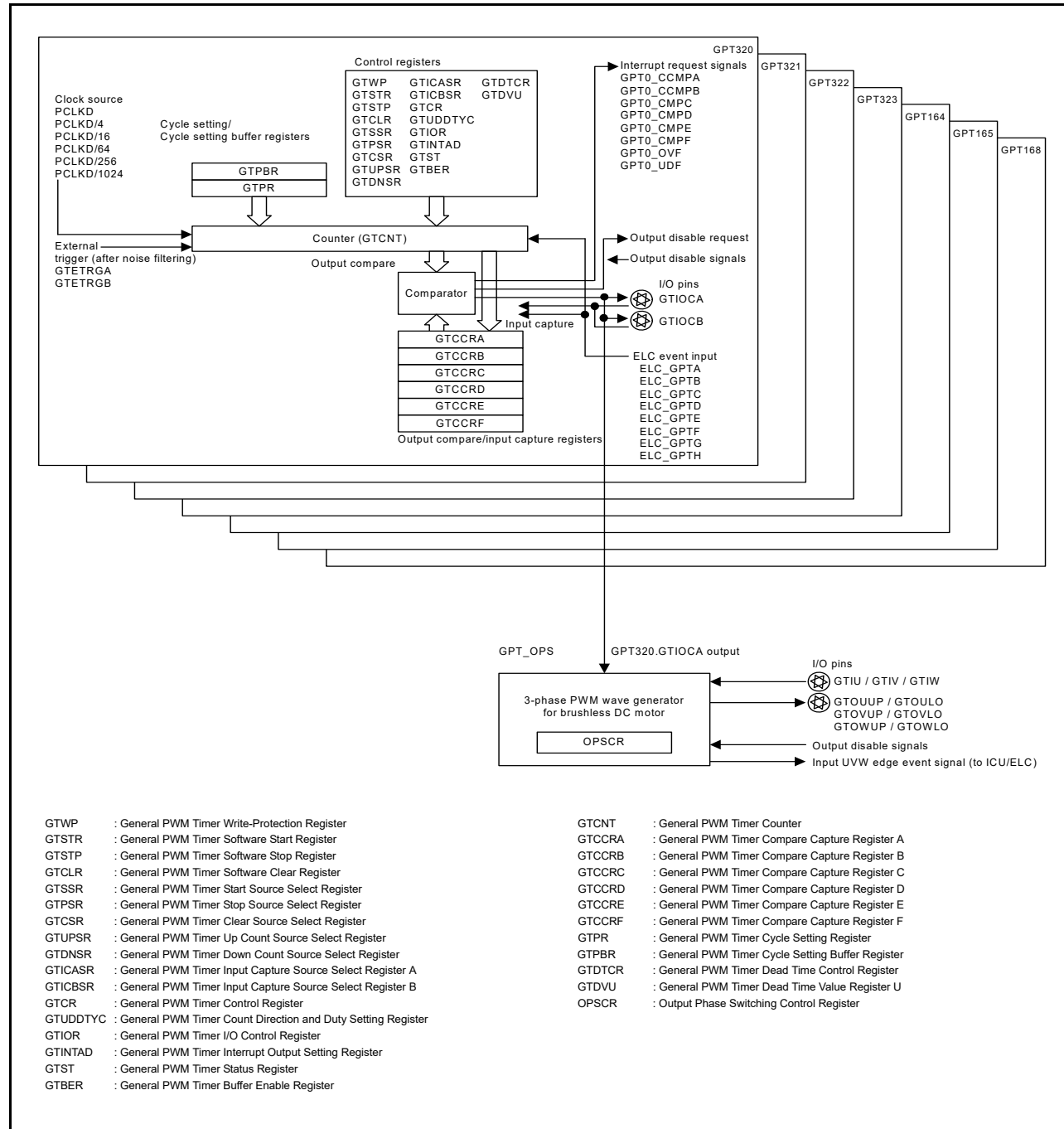
Figure 23.1 GPT block diagram
