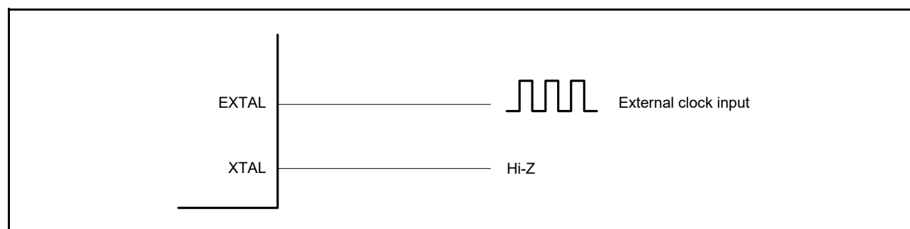
Figure 9.5 Equivalent circuit for external clock
