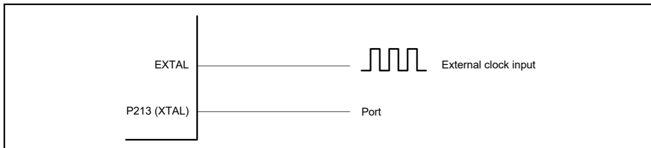
Figure 9.8 Equivalent circuit for external clock
