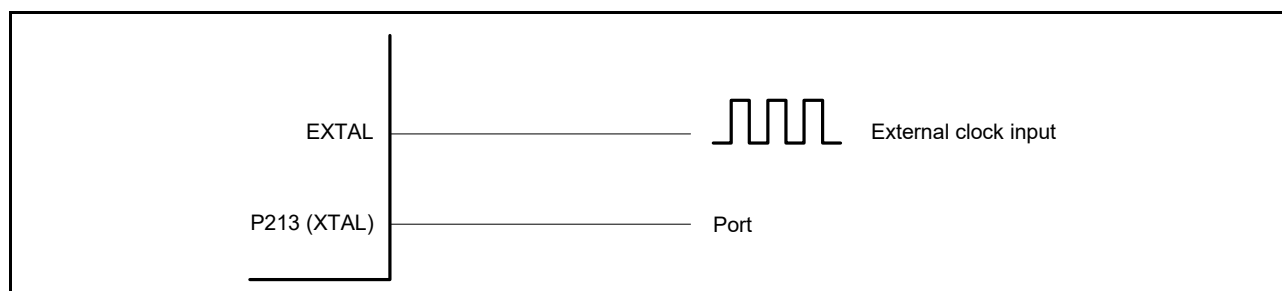
Figure 9.8 Equivalent circuit for external clock
